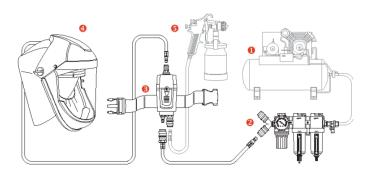
Air is compressed outside of the hazard area (1) and is channelled to a coalescing Filter (2) to be cleaned. From the filter (2), the air passes to the respirator waistbelt (3), where it is regulated to a constant flow. Air then reaches the visor (4) to provide the operator with breathable quality air. It also supplies air to the air tool (5).
